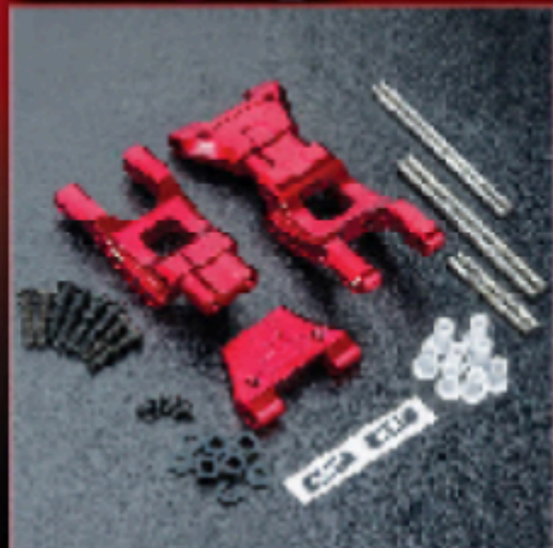
MD Alum. Rear lower arm set (red) MD 铝合金后下臂架 (红)
